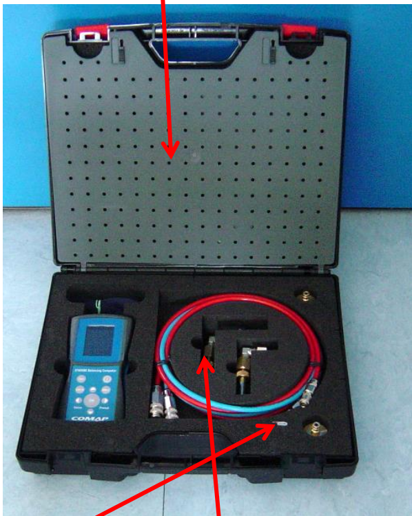
Needle (for TA, Danfoss, Oventrop... valves) and fast connection (Comap) pressure ports adapters
